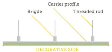
Groove section; spaces of 20 mm
